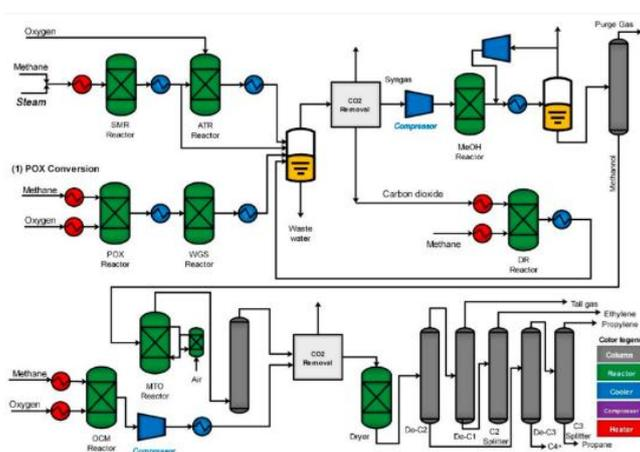
Figure 5. Flowsheet for methane-to-olefins employing SMR, DRM, and POX reforming technologies<sup>31</sup>
