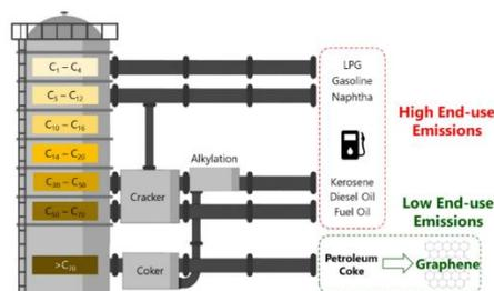
Figure 2. Schematic of Refinery Products.<sup>9</sup>
