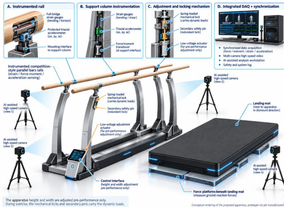
Figure 1. Overall architecture of the proposed instrumented smart parallel bars apparatus. Conceptual schematic only; it does not represent a manufactured prototype.
