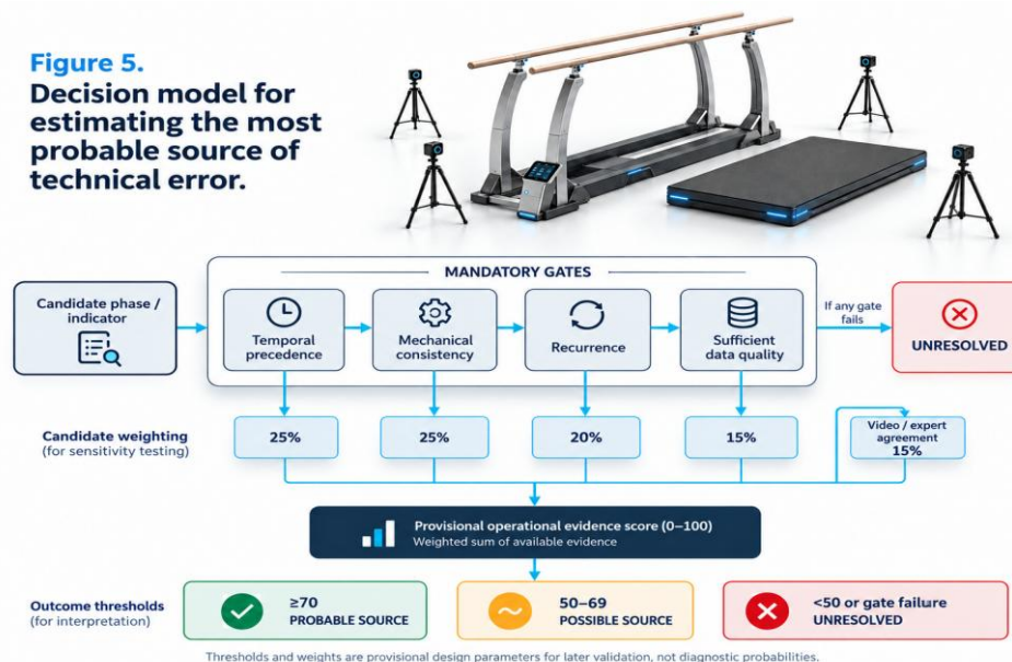
Figure 5. Decision logic for ranking the most probable technical origin while retaining possible-source and unresolved outcomes. Thresholds and weights are provisional design parameters for later validation.
