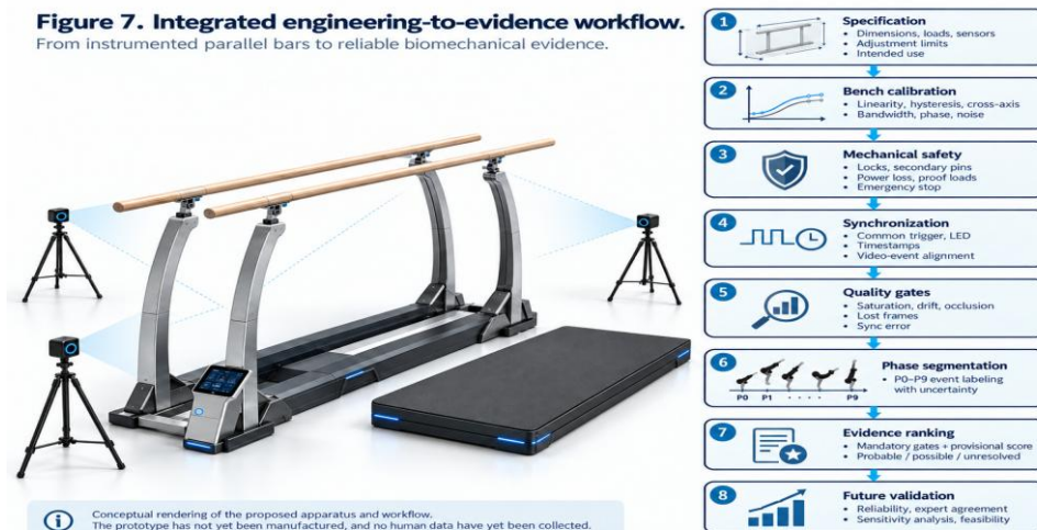
Figure 7. Integrated workflow from design requirements and bench validation to synchronized acquisition, quality gates, evidence weighting, and auditable reporting.
