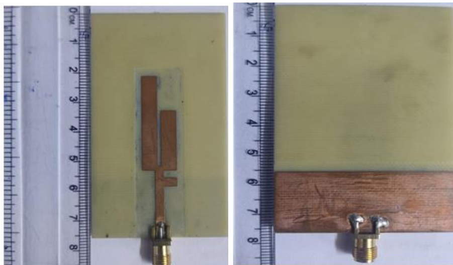
Fig. 11: Top and bottom view of prototype antenna
